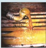
Water contamination on steel mill/ gear
